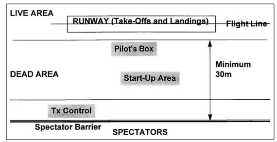
**Figure 3** Typical Display Site Layout
